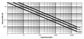
Please note that the figures shown on the previous page are only **typical** figures for standard grade electrolytics at room temperature, please verify readings against expected values for the particular type of capacitor you are testing.
